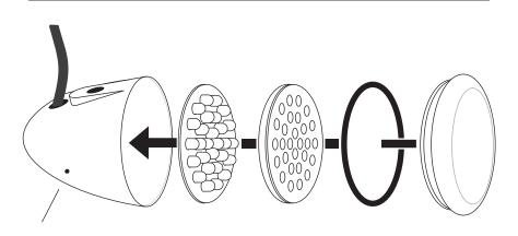
Weephole for Drainage: This should be located at the bottom of the light when mounting. Each package contains a left and right bullet light, be sure your weephole is facing downward for proper drainage.
