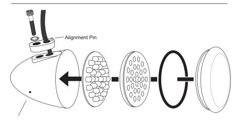
Weephole for Drainage: This should be located at the bottom of the light when mounting. Each package contains a left and right bullet light, be sure your weephole is facing downward for proper drainage.
