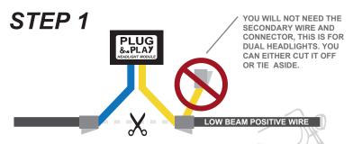
LOCATE THE LOW BEAM POSITIVE WIRE AND CUT IT INTO 2 PEICES. USE FIRST CONNECTOR ON YELLOW AND BLUE WIRES. STRIP 1/2" FROM YOUR LOW BEAM POSITIVE WIRES. SQUEEZE CONNECTORS AND PLACE STRIPPED WIRE IN, LET GO AND TUG THE WIRE TO VERIFY A SECURE CONNECTION.
