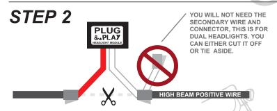
LOCATE THE HIGH BEAM POSITIVE WIRE AND CUT IT INTO 2 PEICES. USE FIRST CONNECTOR ON RED AND WHITE WIRES. STRIP 1/2" FROM YOUR HIGH BEAM POSITIVE WIRES. SQUEEZE CONNECTORS AND PLACE STRIPPED WIRE IN, LET GO AND TUG THE WIRE TO VERIFY A SECURE CONNECTION.
