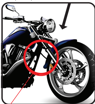
Mount photo optic sensor under fairing pointing downward.
