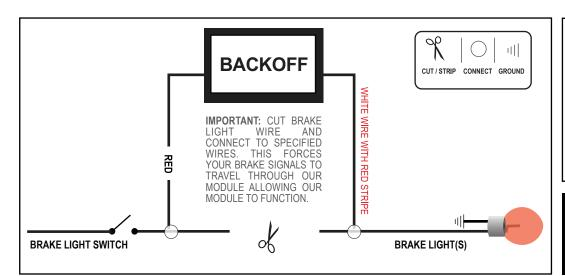
Once installed, The original BACKOFF module will emit 3 short brake light flashes and then one long flash and it repeats. The signal automatically repeats itself as long as the brake lights are on. This pattern is not random, but has been selected because of its ability to retain following drivers attention.
